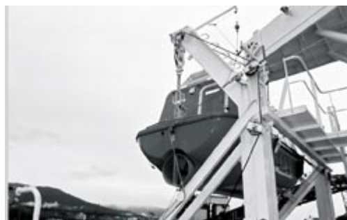
Photo 6. After view of lifeboat, showing davit, gripe arrangement around bollards, suspension ring, hook, and hatch
