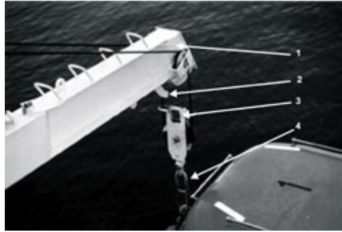
Photo 4. 1. Davit head, 2. Horn, 3. Eye in floating dock, 4. Suspension ring
