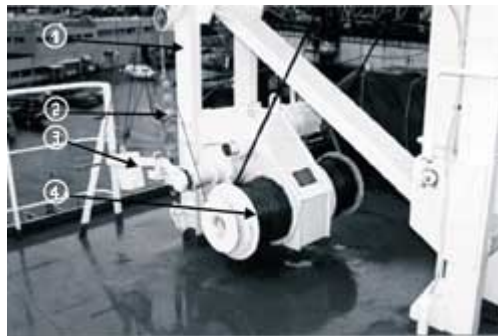
Photo 5. 1. Frame, 2. Gripe, 3. Dead man's handle (winch brake), 4. Winch drum
