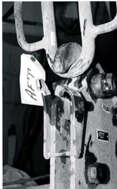
Photo 16. Damage to the after retaining latch
