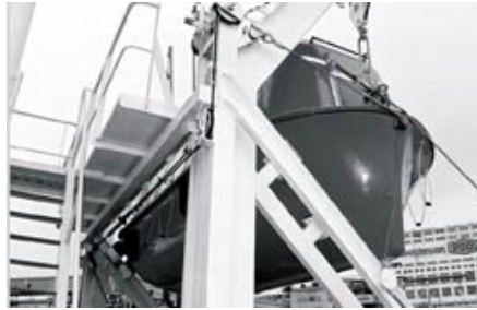
Photo 8. Forward view of lifeboat, showing davit, gripe arrangement around bollards, suspension ring, hook and hatch
