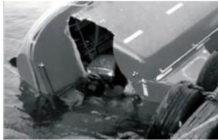
Photo 15. Damage to the stern of the lifeboat
