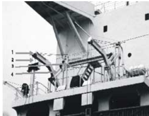
Photo 3. 1. Davit, 2. Falls, 3. Embarkation platform, 4. Frame
