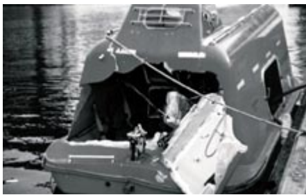
Photo 14. Damage to the stern of the lifeboat
