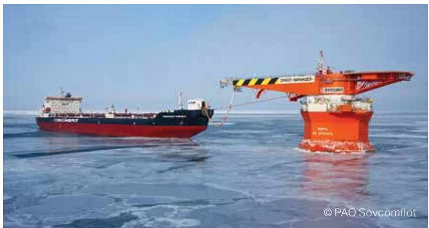
Example of a Category A ship – TIMOFEY GUZHENKO, Ice Class ARC6 icebreaking tanker
