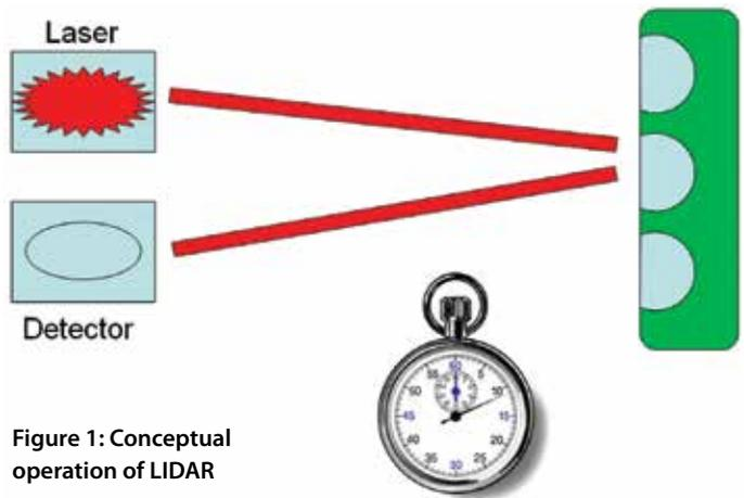
Figure 1: Conceptual operation of LIDAR
