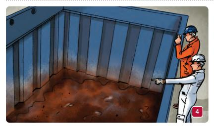
The master should observe the start of loading and look and listen for signs of splattering (muddy splashing) of the cargo on tank tops and bulkheads. This is an indication that the cargo may be in a fluid condition.
