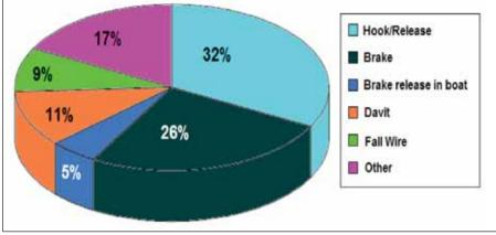
▲ Table 1: Component failure: from OCIMF survey, 1994
