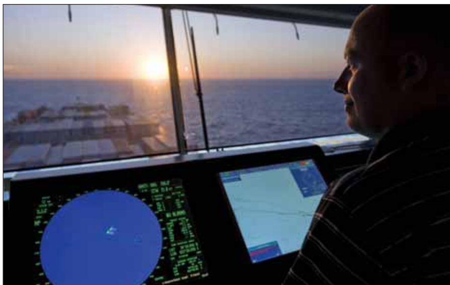
▲ It is vital to correlate ECDIS with other input, such as radar
