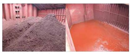
Iron ore fines before and after liquefaction.
