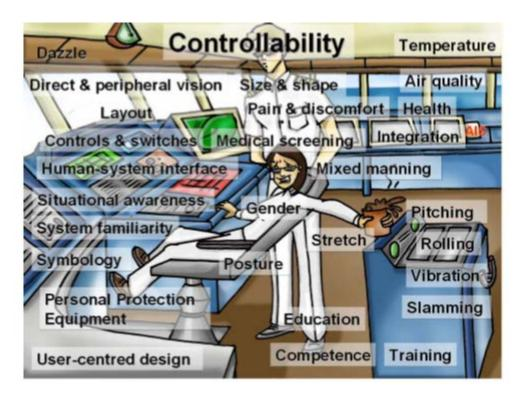
This cartoon shows a state of the art ship control centre comprising of an Integrated Bridge System (IBS). While it seems that some attention has been given to the layout of the IBS (by the equipment manufacturer) there has been no user input to the design of the bridge space itself. The Master is British - at 6'5" (1981 millimetres) he has problems of:
