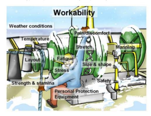
This cartoon shows a single Asian crew member is on the fo'c's'le tending the windlass at the same time as he is taking in a tug's line. It is very wet and cold with a wind chill factor that makes for freezing conditions. The problems are:
