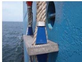
Fig 1 Securing points inset to the vessel's hull are fairly common [Kevin Vallance]
