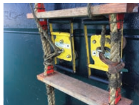
Fig 4 Improperly positioned magnets – they should be outside the ladder [Giuseppe Raffa]
