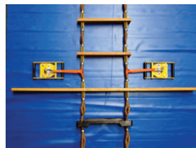
Fig 3 Hull magnets in use, positioned correctly [Marine Safety Supplies]
