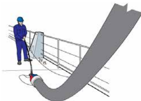
Fig 7-55. Laying out the hoses on deck aft of the rig
