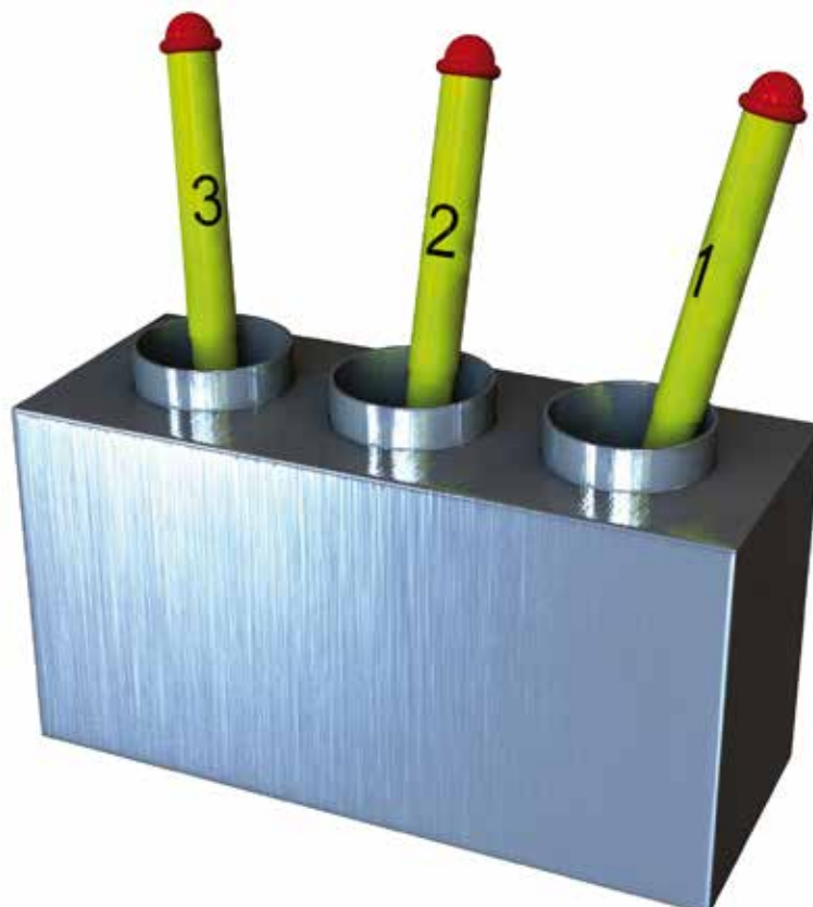
Fig 7-17. Example of locally manufactured gunline container stowage
