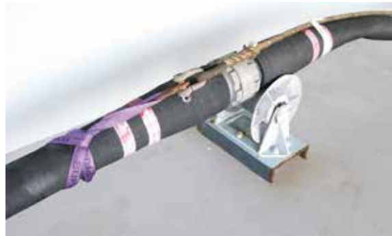
Fig 7-79. Heaving-out rope secured to knuckle
