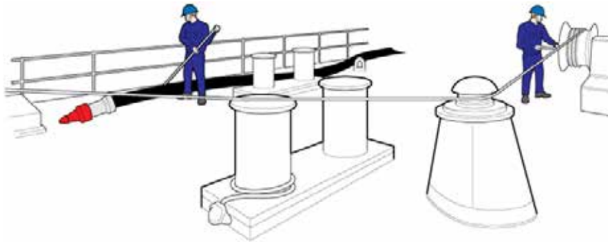
Fig 7-83. Using a capstan bar to ease the hose end outboard
