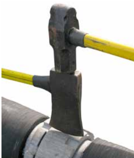
Fig 7-92. Disconnecting a seized hose
