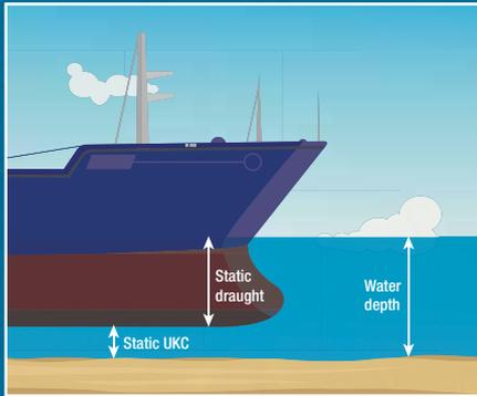
◀ **Figure 1 – Static UKC:** static draught is taken to be the maximum of fore and aft draughts
