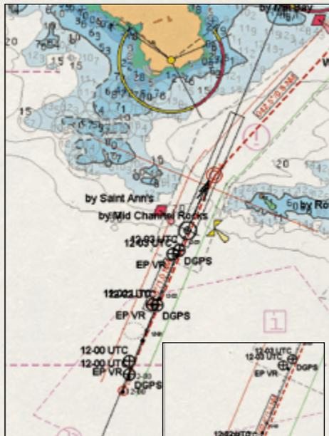
Position fixing using LOPs employed for verification of GNSS positions
