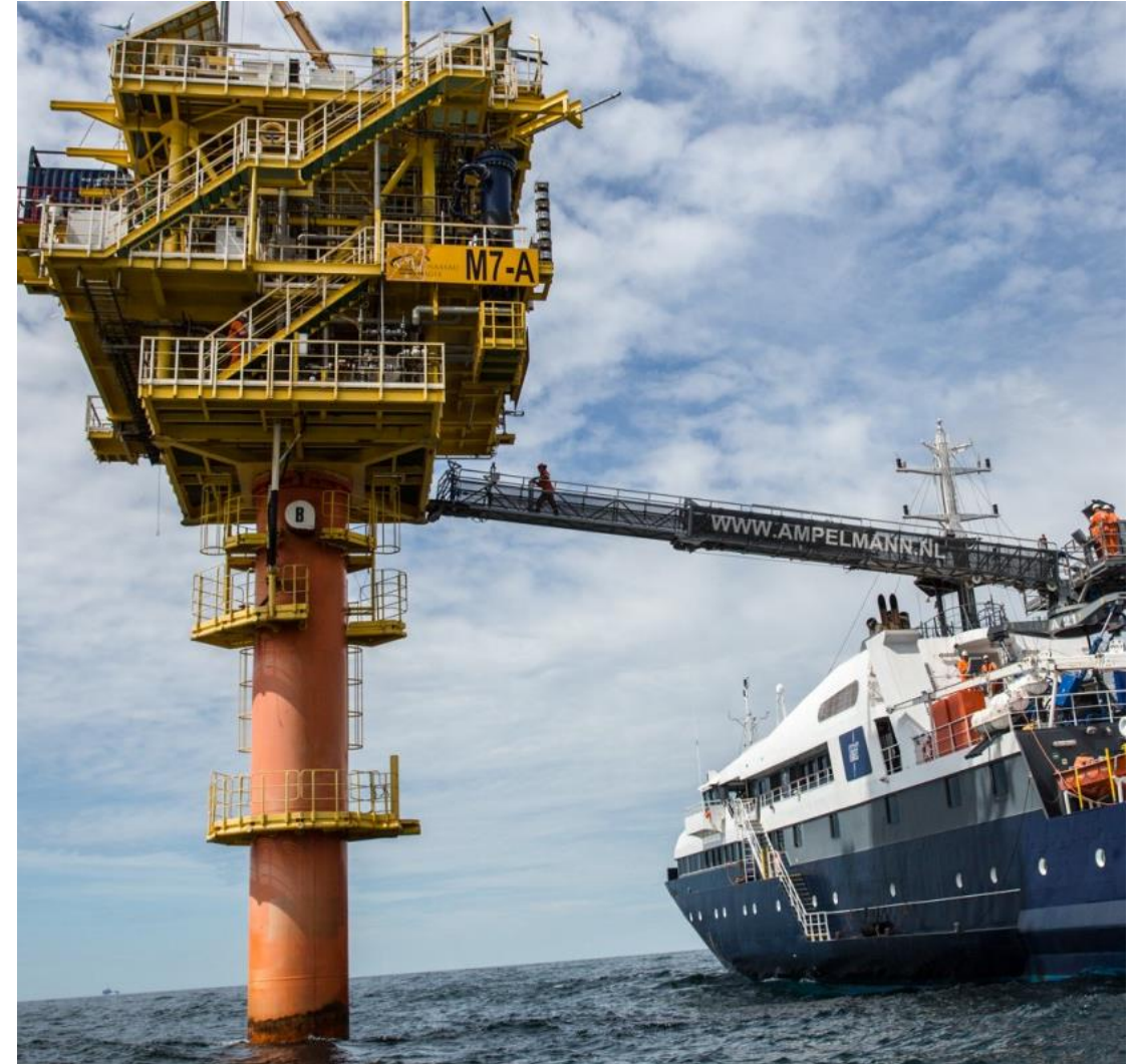
Walk to Work solution – a vessel with Ampelmann offshore personnel transfer system (Source: ampelmann.nl)
