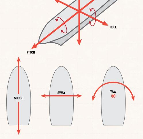
place across two planes: the horizontal and vertical. On the horizontal plane, the vessel is subject to surge (forward and aft), sway (port and starboard) and yaw (around the horizontal axis)
