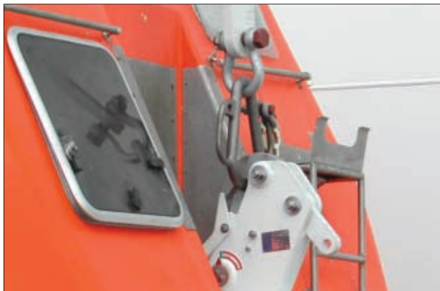
▲ Hook replacement: LRH 12 on the Celebrity cruiseship Millennium
