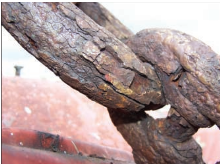
▲ These photographs, a small sample of the many sent to Schat-Harding by the company's engineers, show what can happen if lifeboats and hooks are not properly maintained.
