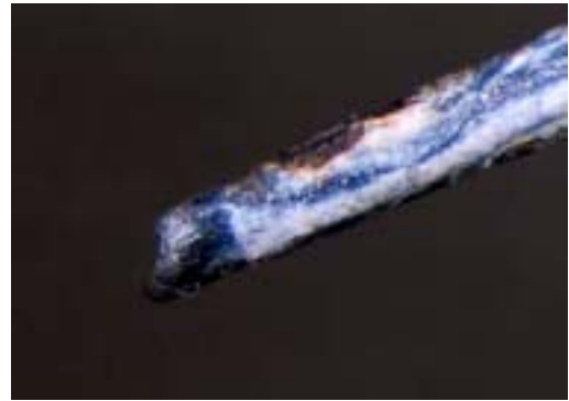
Figure 9. Strand outer wire also showing localised necking.
