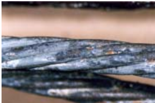
Figure 3 (top left). Illustrates the extent of the corrosion damage to the outer wire strands adjacent to the fracture.
