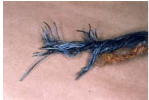
Figure 7. Inner wire strands at the point of failure.
