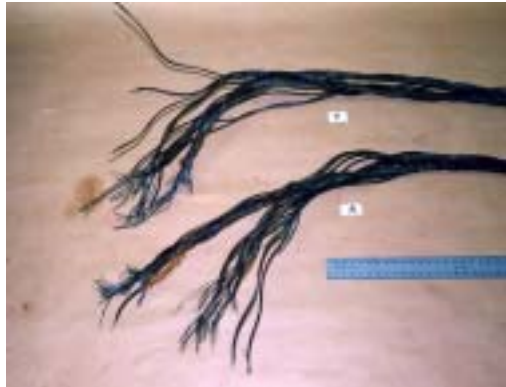
Figure 6. Forward and aft davit ropes at the point of failure. Note the splaying of the outer strands.
