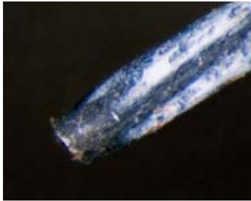
Figure 8. Ductile 'necking' of a strand core wire. Classic cup-cone style tensile fracture.
