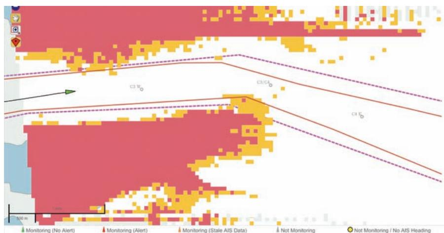
Figure 5: Chart overlay (web-view) showing no-go areas and warning areas at a safe speed
