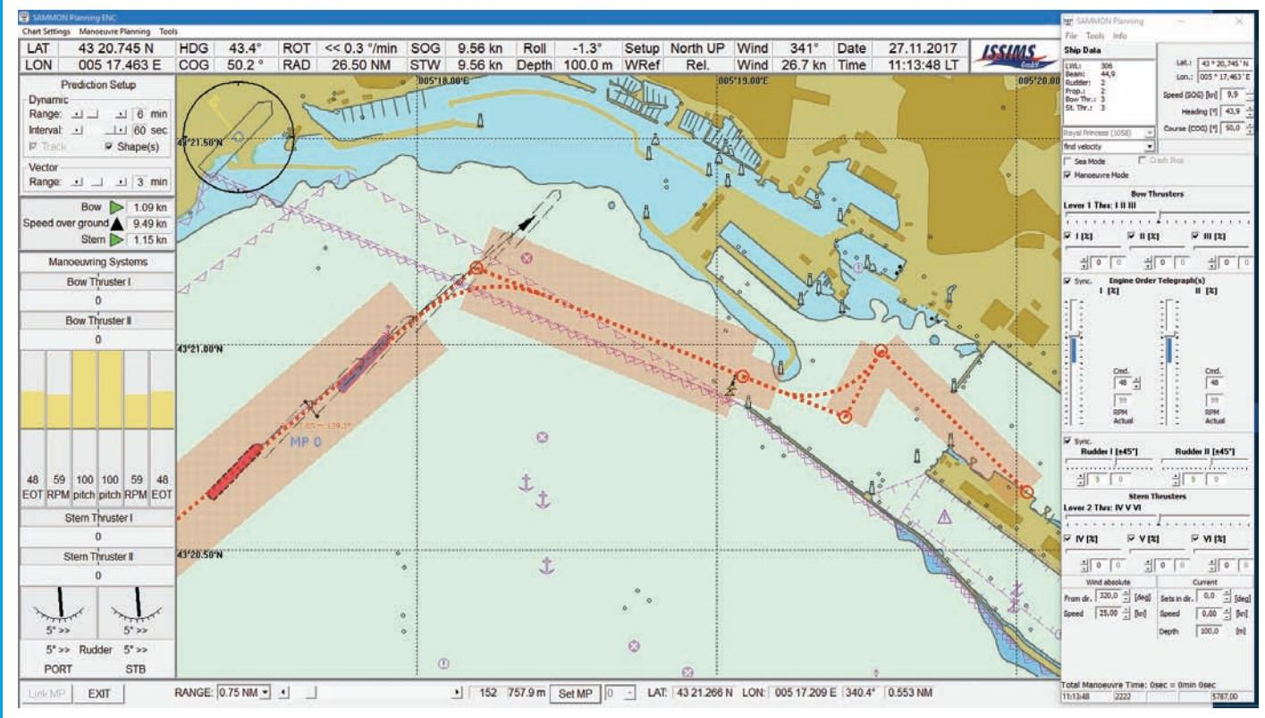
Figure 4 SAMMON planning module: route plan imported from NACOS (red dotted lines and circular segments) and start of manoeuvring planning at manoeuvring point MP0 (red shape); predicted manoeuvring track for 6 min (black dotted contours every minute) and shifted position for the next MP (blue shape with red frame)
