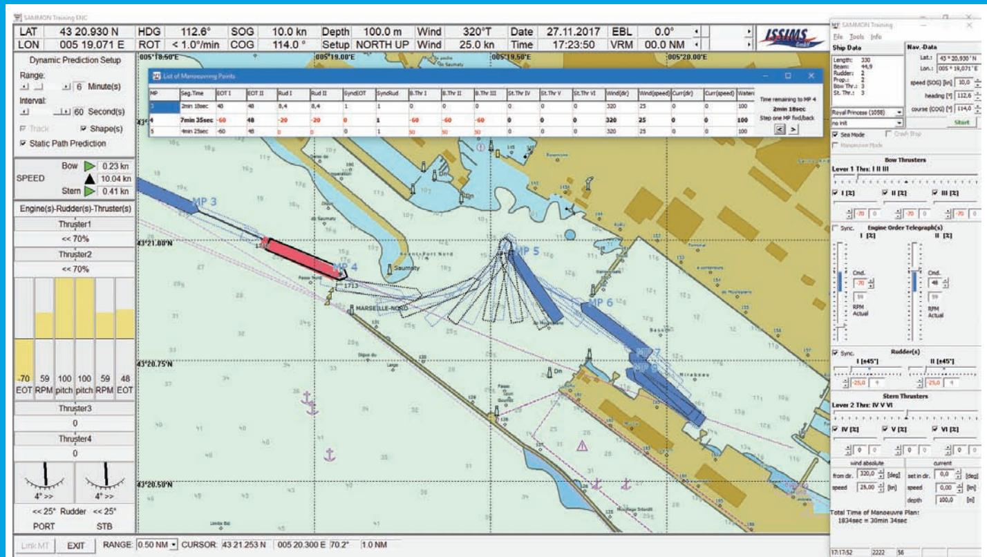
**Figure 4 SAMMON Trial & Training Tool with multiple predictions: Real time simulation and manoeuvring prediction are integrated into ECDIS. The display compares Full Dynamic Predictions (black dotted ship contours) and the simple static prediction (magenta curve) together with planned manoeuvring track (blue line and ship shapes)**
