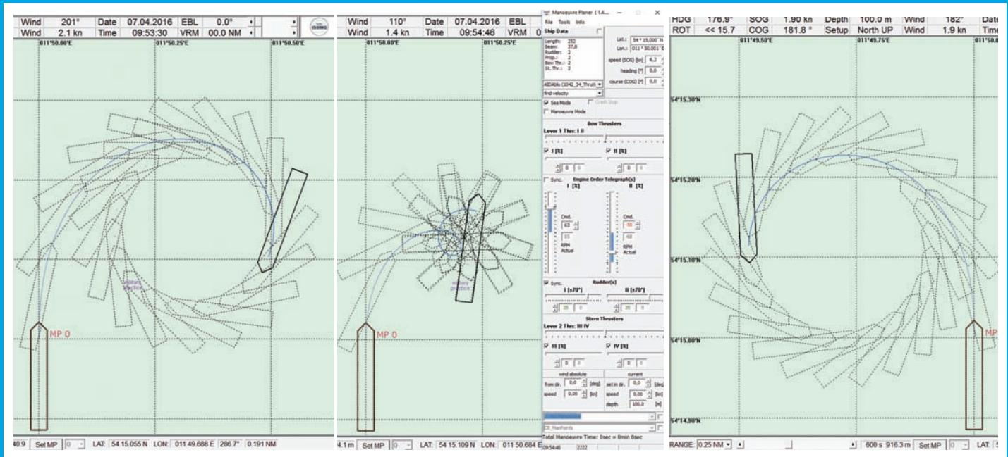
Figure 2 Comparison of turning manoeuvres from an initial speed of 6.2 knots with constant speed
