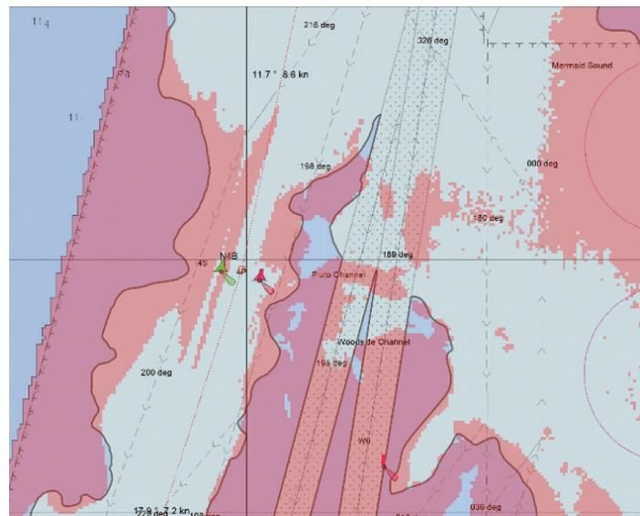
Figure 8: Actual PPU displays on Panasonic Toughbook during transit (2016) with detailed sectional view
