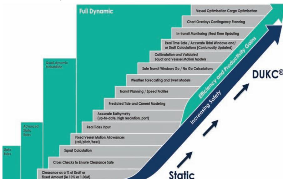
**Figure 2: Steps to a safer underkeel clearance management system**
