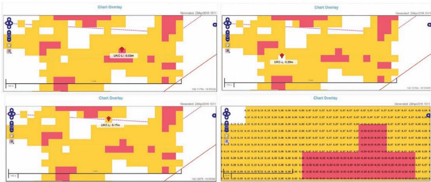
Figure 7: Interrogation of cells (drill-down) to see actual UKC clearances per computed cell
