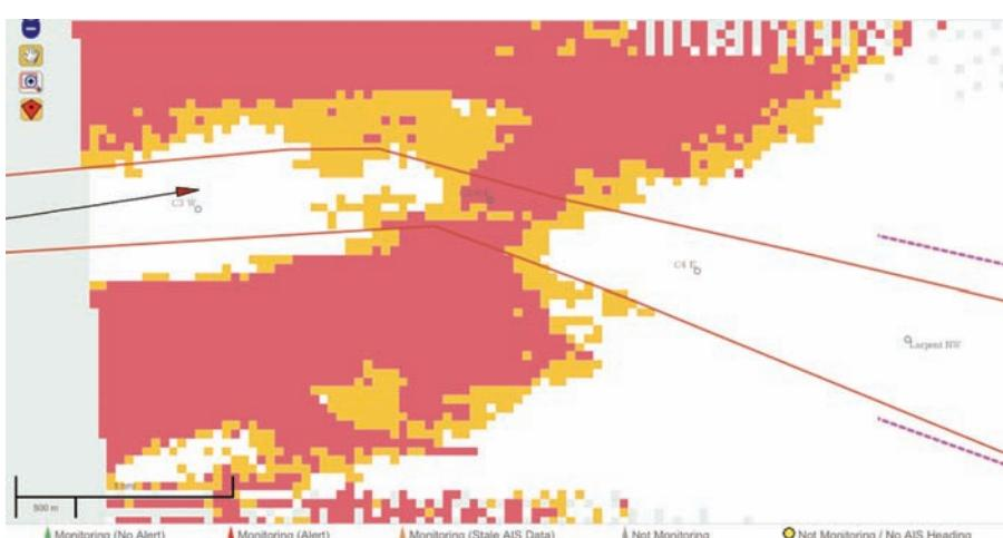
Figure 6: Chart overlay (web-view) showing no-go areas and warning areas at an unsafe speed
