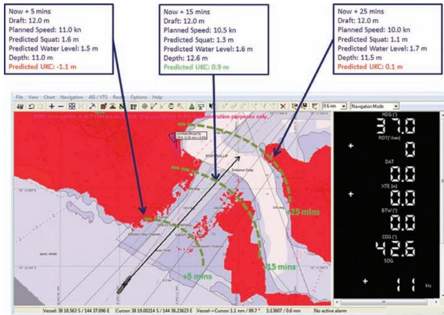
Figure 4: Dynamic overlay with predictive calculations for the transit
