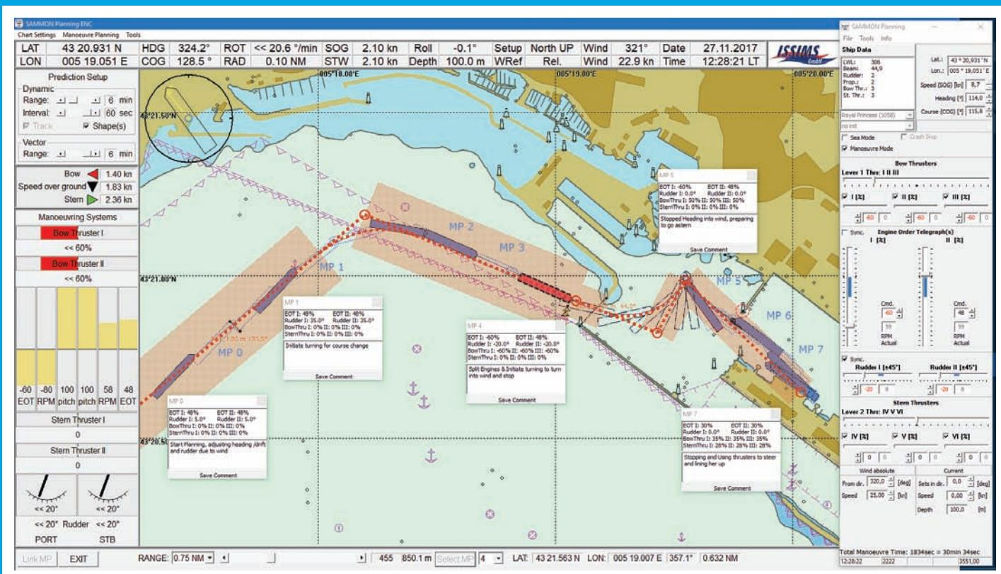
Figure 5 SAMMON planning module: complete manoeuvring plan from SAMMON planning module (blue line and shapes), based on route plan (red dotted lines) imported from NACOS
