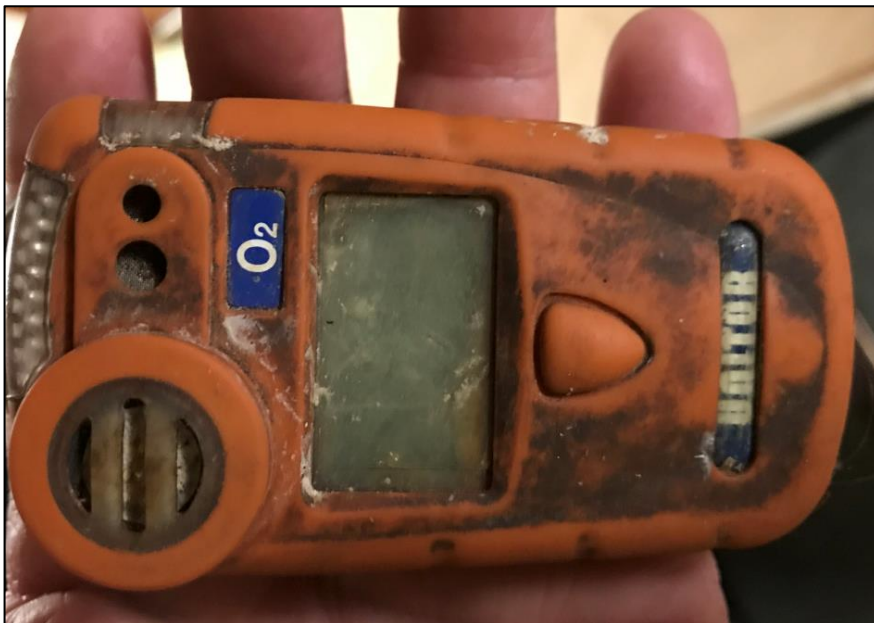
Figure 5: The oxygen detector in use at the time of the accident was of the type Unitor OXY-MATE C. Photo: AIBN
