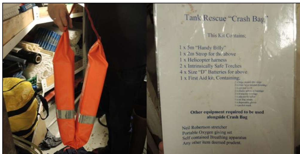
Figure 8: The rescue equipment included a lifting strop. The equipment was kept in a storeroom by the entrance to the forward starboard silage tank. Photo: AIBN
