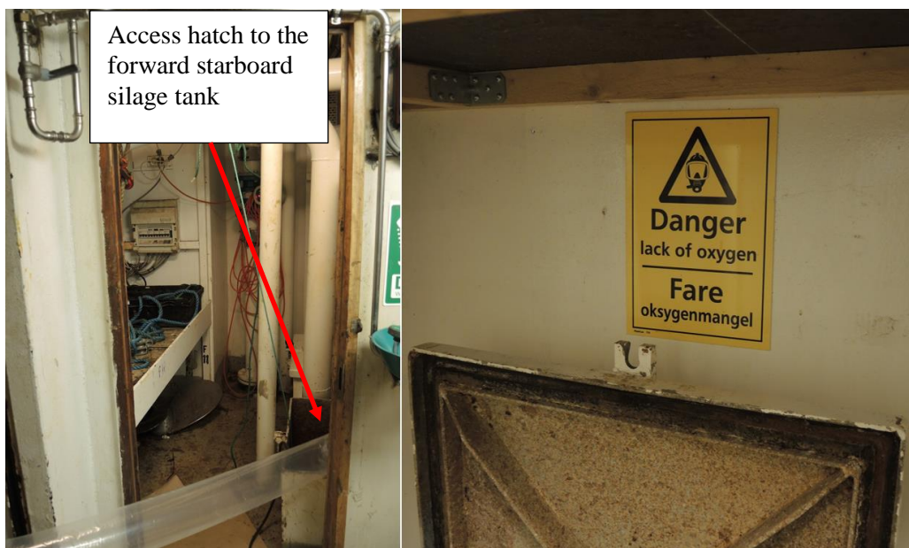
Figure 4: The access hatches for the two forward silage tanks were located forward of the factory, inside a confined space in the vessel's interior. There was a sign above the hatches with the text 'Danger lack of oxygen'. Photo: AIBN
