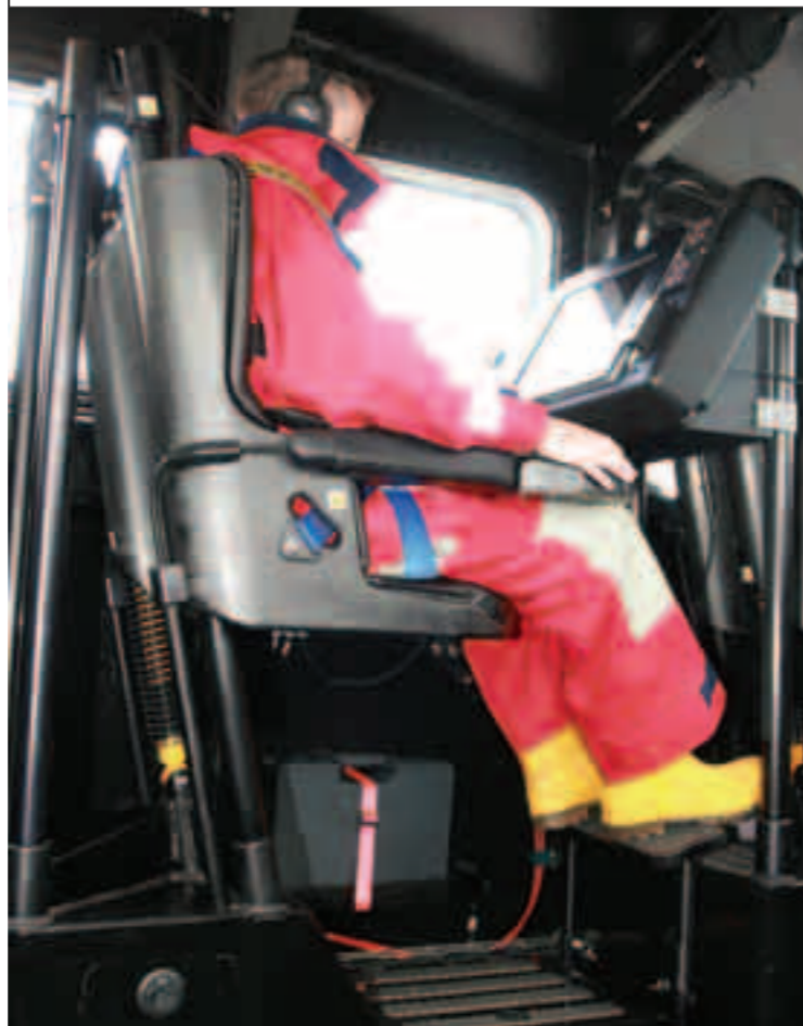
Safely seated, the mechanic can monitor, operate and control onboard systems © RNLI
