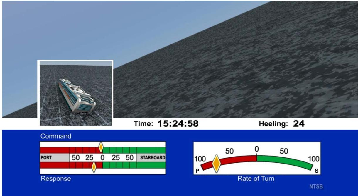
This screen shot from the *Crown Princess* animation shows the view from the bridge at the full heeling angle. The ship at full heel is shown in the inset. At the bottom of the screen are the rudder command indicator, the response indicator, and the rate of turn indicator.
