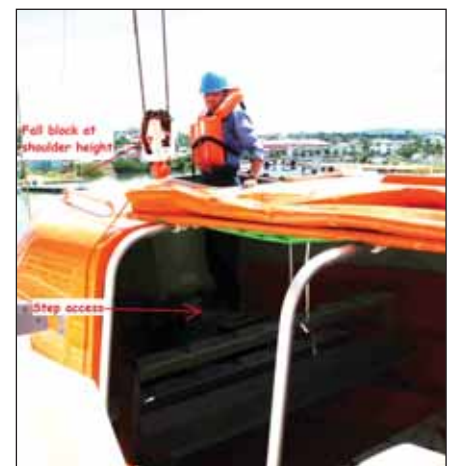
▲ Forward hook access
