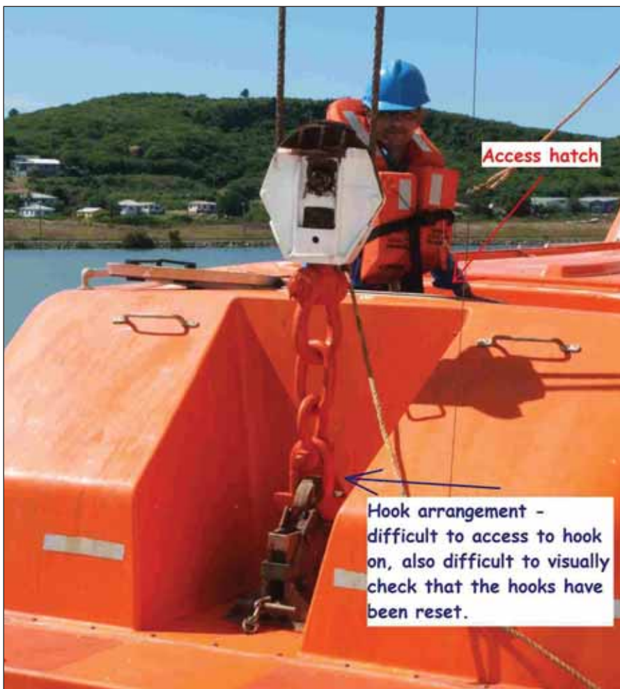
▲ These pictures show difficulties in hook access and visual checking
